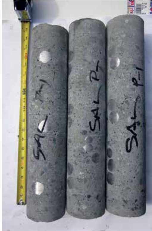
Fig. 3: Cores retrieved from Type 1 preconstruction test panel
