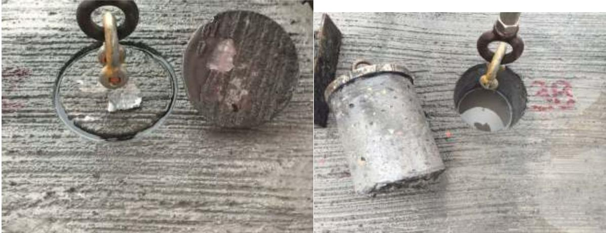
Picture of glue plane failure
